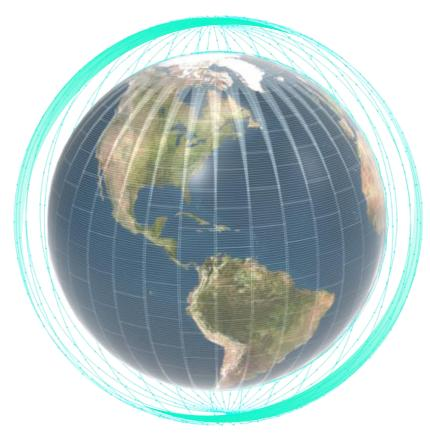
882 LEO satellites will operate at an orbit of 1,200km above the earth
