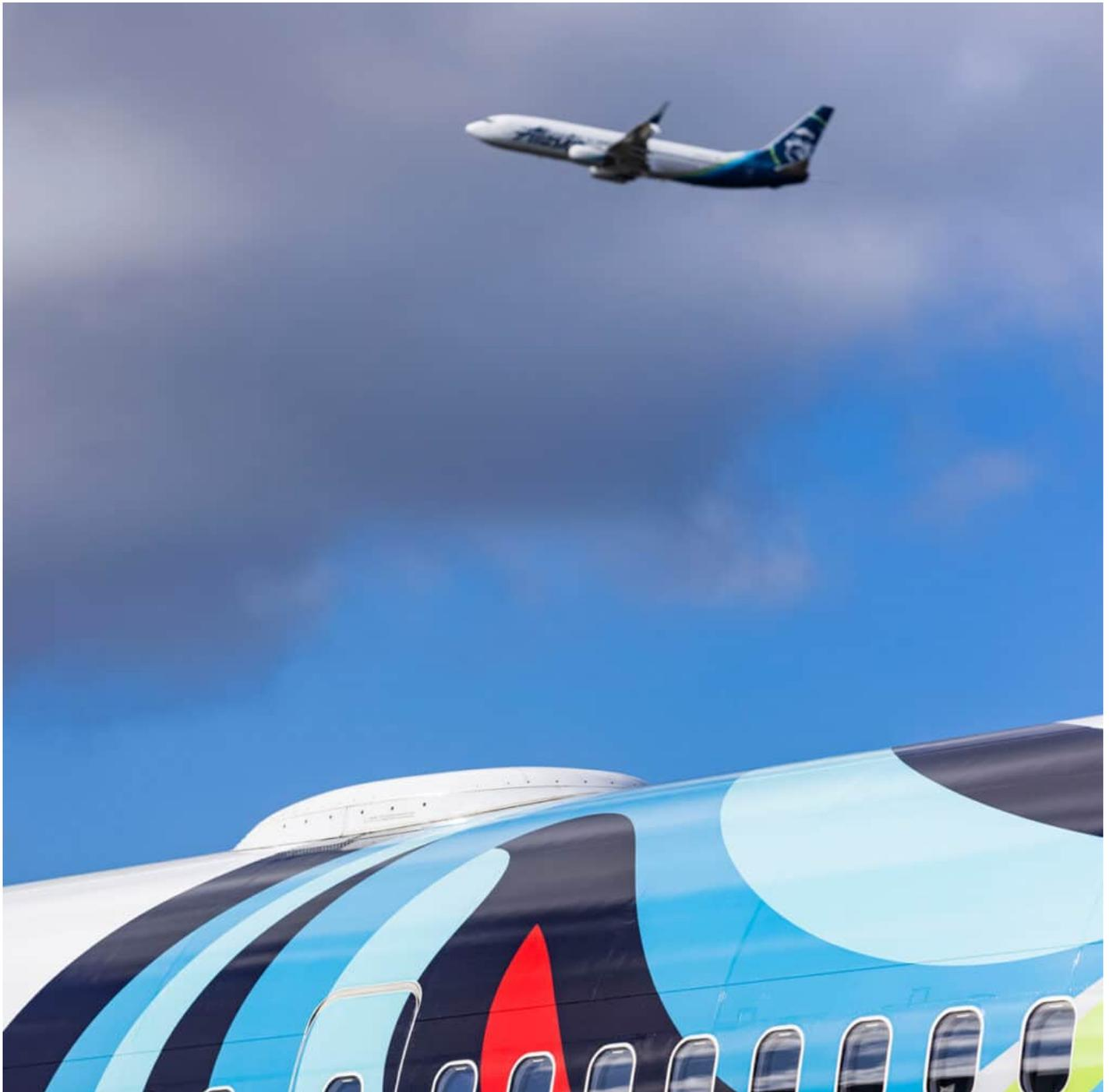
Boeing 737MAX installed with 2Ku on top, in the foreground, and another, yet to be installed, flying in the background (courtesy: Alaska Airlines).
